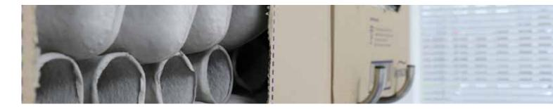
Testing to determine whether using pulp disposal units for single-use sanitary products caused any obstruction in the waste pipes.
