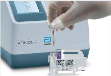
Place the test cartridge in the analyzer and close the lid. The processing starts automatically.
