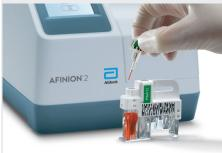
Place the test cartridge in the analyser and close the lid. The processing starts automatically.
